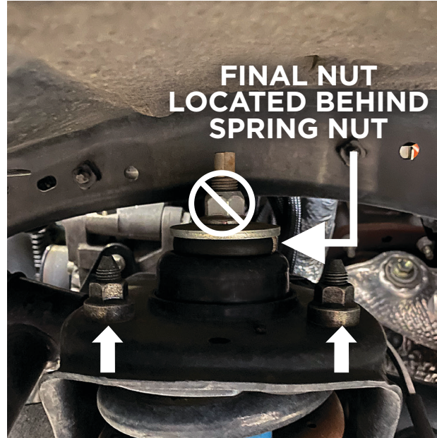
Fig. 2: DO NOT remove the center nut. Remove the top hat nuts (arrows).
