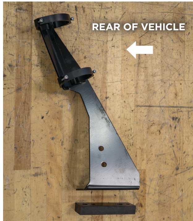
Fig. 10: Front reservoir bracket orientation.
