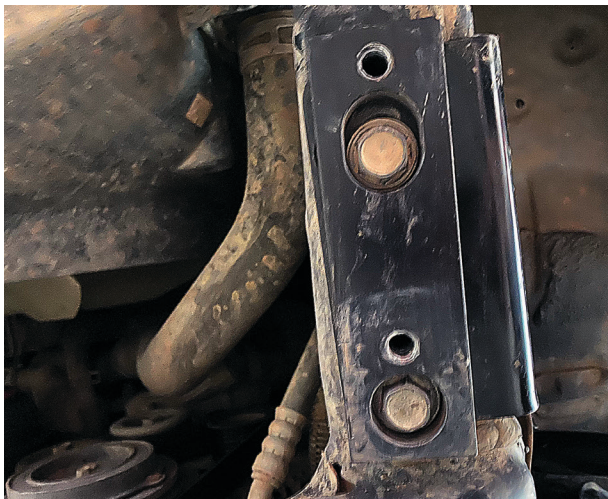
Fig. 5: Sway bar relocation spacer (bottom view).
