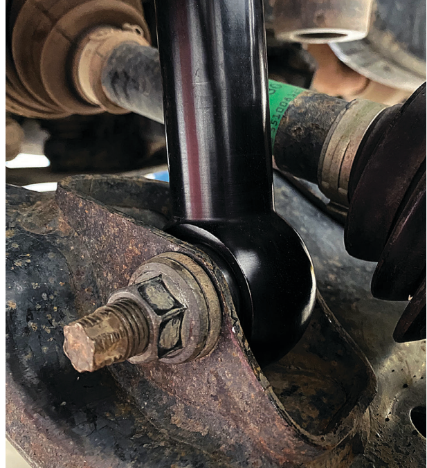
Fig. 4: Installed lower shock bolt.
