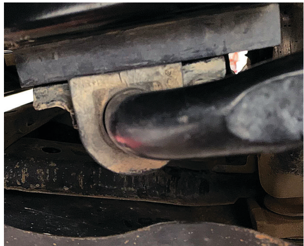
Fig. 6: Sway bar relocation spacer (side view).
